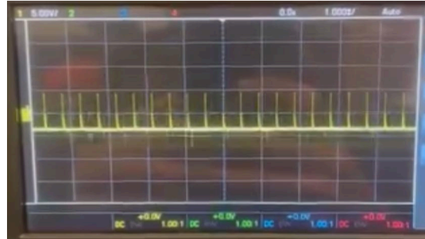
Figure 5: Oscilloscope Reading for Reversed Motor
